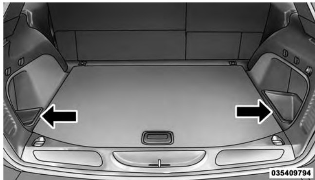
Rear Storage Bins
