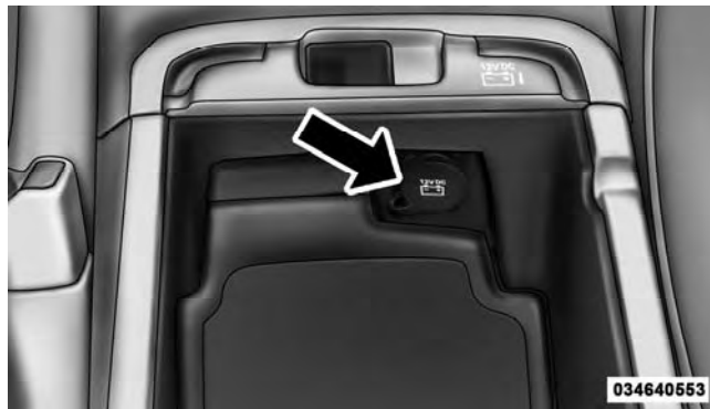
Front Center Console Outlet
