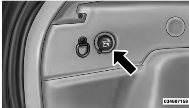
Rear Power Outlet
